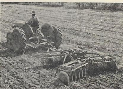
DISC HARROWS — Tandem or single — angle of discs hydraulically controlled.
